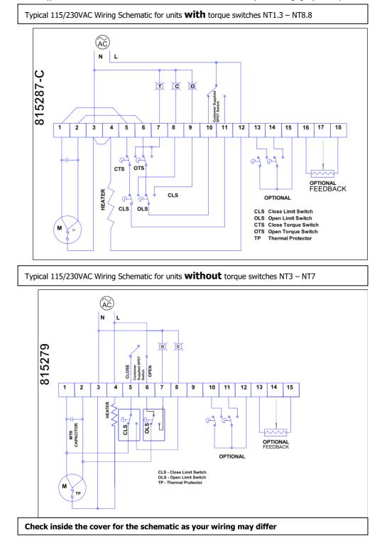
The wiring diagram shown below is typical. The SPDT Automatic Control switch and some of the other items (i.e. indicating lights) are not provided and must be wired by the customer.
